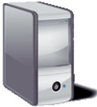
**Computer tower:** The case that holds all the electronic components of the computer. On the outside of the case is where you can plug in headphones, microphones and USB devices. These ports are usually found on the front of the case. The ports for network cables, printers and power cords are usually found in the back.
